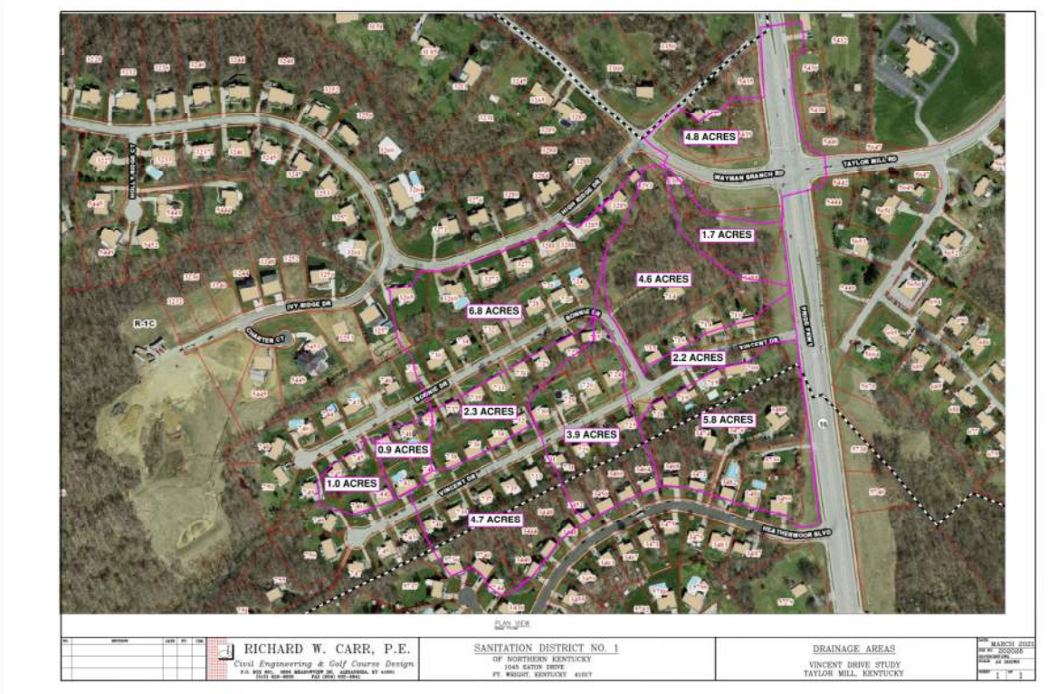
Figure 2 – Delineation of drainage areas
